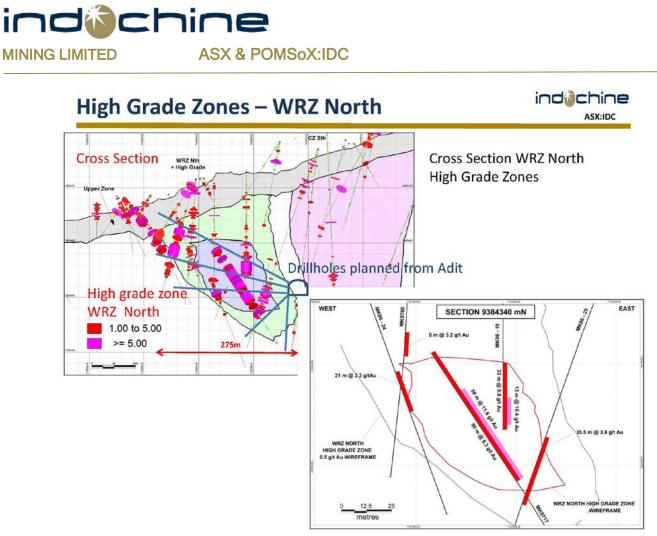
Figure 4: Cross section of high grade gold zone (WRZ North) with adit location and drillholes.
