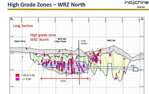
Figure 3: Long section of high grade gold zone (WRZ North) with adit location.
