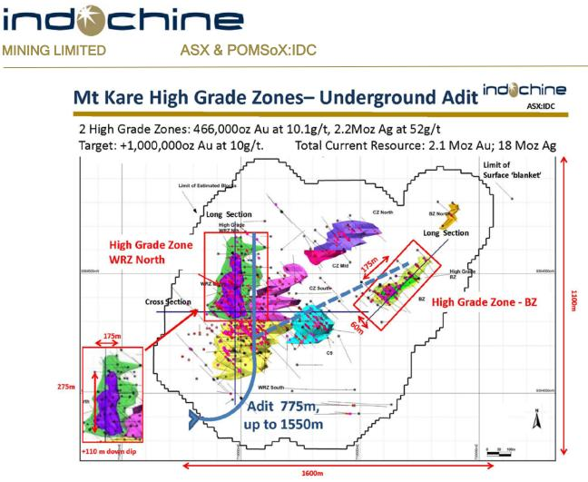
Figure 2: Plan view of Mt Kare with high grade gold zones (WRZ North and BZ) with adit location.
