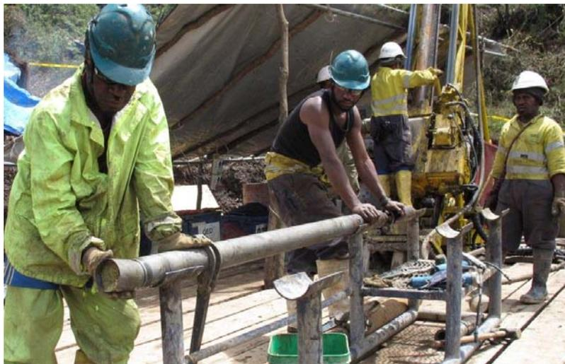
**Figure 6: Recovering drill core at drillhole 126SD12**
