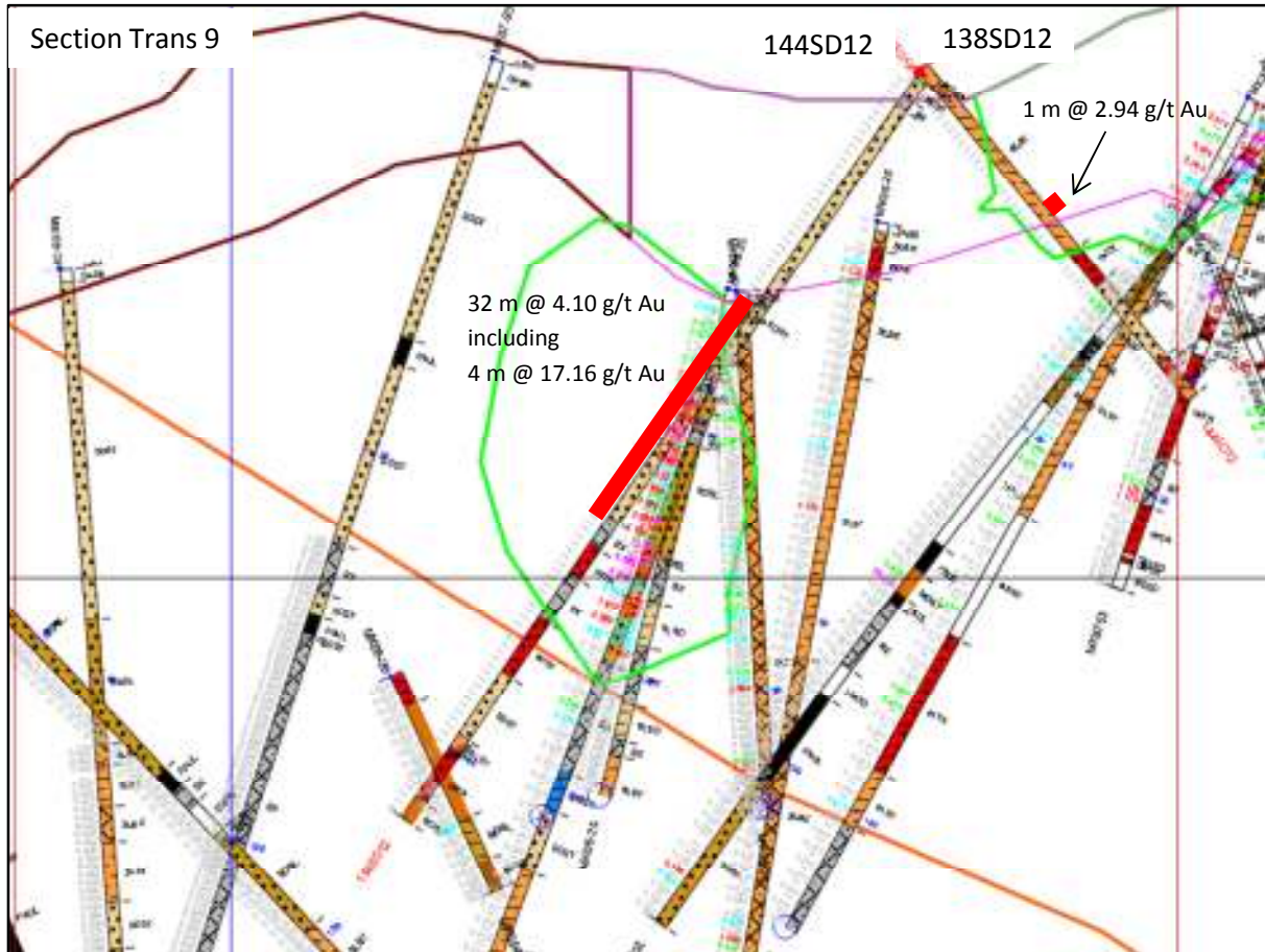
Figure 5: Cross-Section – WRZ resource block with past and new drill assay results (red bars) from 144SD12 and 138SD12
