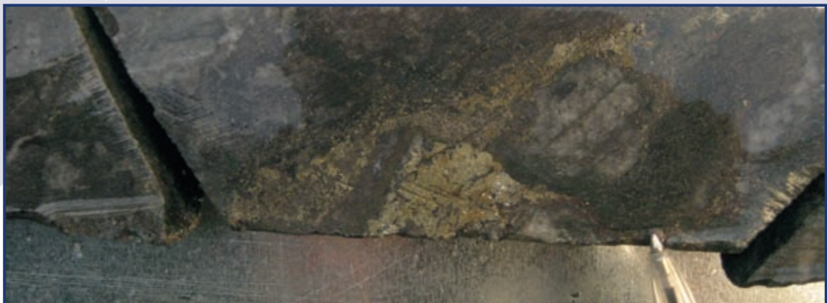
Plate 3: Breccia and Sulphide Mineralisation at 110.0m in STN07 at Elephant Prospect.
