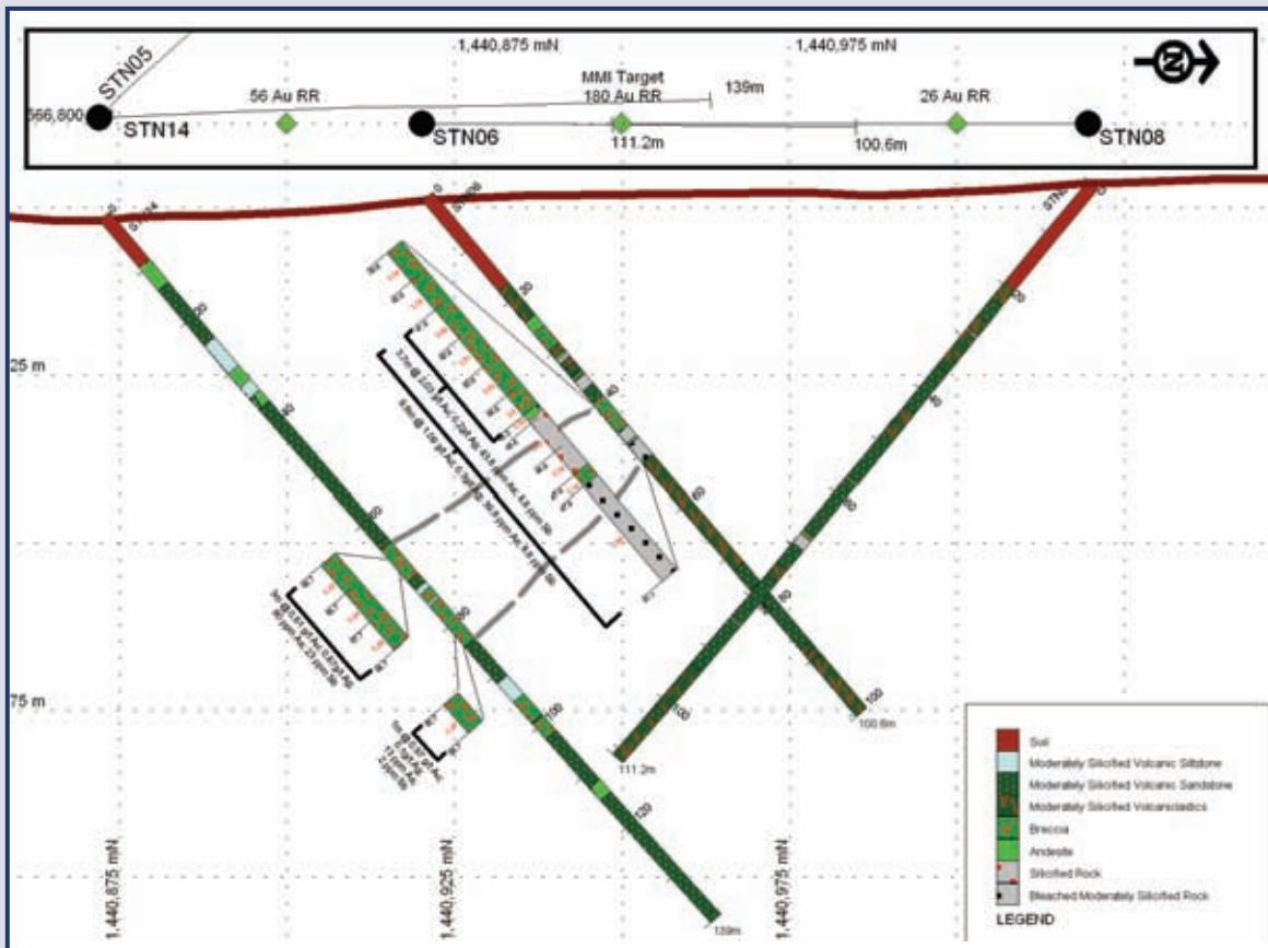
Figure 16: Cross section Through STN06, 08 & 14.
