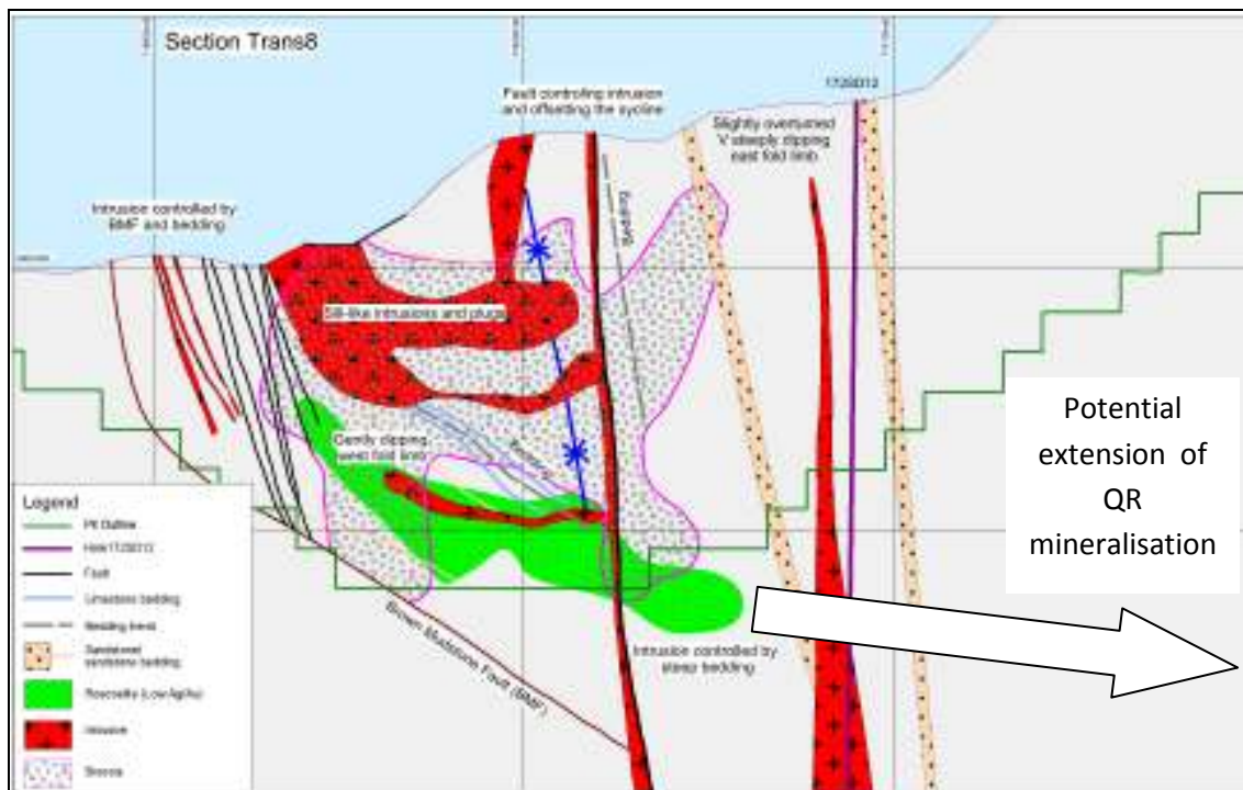
Figure 1: Quartz-roscoelite (QR) mineralisation in the WRZ and potential extensions
