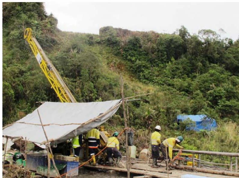
Figure 3: Drill rig at 125SD12 in the WRZ resource zone
