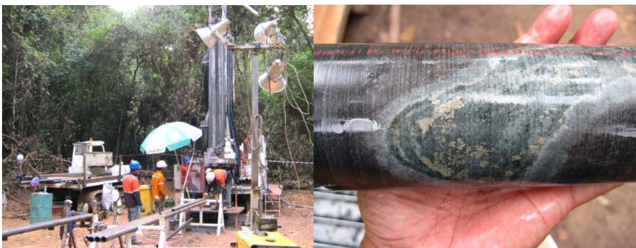
Kratie North, Cambodia – Drill rig; Drill core with quartz-pyrite veins in fresh rock
